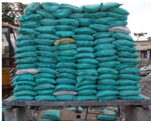
Fig.9 Test load with sand bags for slab MO3
