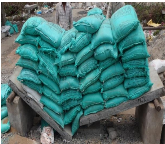
Fig.7 Test load with sand bags for slab MO1
