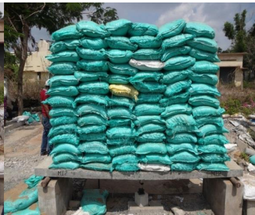
Fig.6 Test load with sand bags for slab MI2
